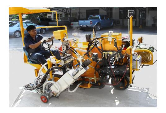
The Powermaster 180 is the smallest ride-on thermoplastic extrusion machine available. A fully automatic machine with many work possibilities. Small jobs are easy as the material can be mixed and melted in the tank.
