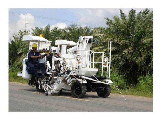
The Highwayman is the perfect choice for medium to large lining works. The machine is equipped with extrusion which can be used on either side of the machine.
