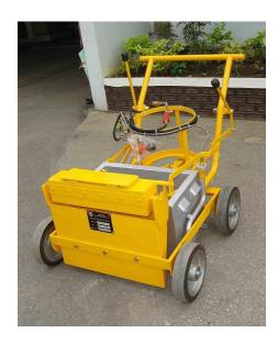
The Unimark Pedestrian Crossing Machine is a hand pull machine applying screed thermoplastic panels in widths according to individual specification but typically 70 cm wide. The propane gas heated tank will apply one panel per fill at 3 mm thick. An adjustable glass bead dispenser is fitted for instant retroreflectivity. The machine is designed to give very neat single application panels for professional finish to pedestrian crossings.
