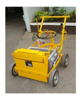
The Unimark Pedestrian Crossing Machine is a hand pull machine applying screed thermoplastic panels in widths according to individual specification but typically 50 cm wide. The propane gas heated tank will apply one panel per fill at 3 mm thick. An adjustable glass bead dispenser is fitted for instant retroreflectivity. The machine is designed to give very neat application single panels for professional finish to pedestrian crossings.
