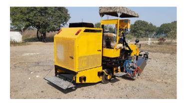
The UNIMARK POWERMASTER 450 EX is the next generation extrusion road marking machine. It is a 4 wheel machine with enhanced tank capacity & heating capability.
