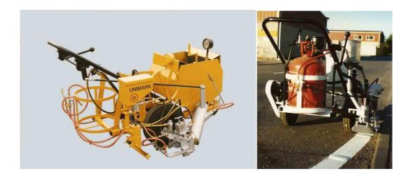
The machine will apply the proven and long lasting original raised rib thermoplastic profiled line. The unique and original Unimark pneumatic system gives automatic rib spacing on the base line in a single application. The profile laying shoe is connected to the delivery tube with our quick change rotary connection which also allows the shoe to follow any road contour deviations. With a tank capacity of 65
