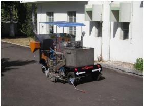
**Engine:** Briggs & Stratton Electric Start, 13HP Petrol driven, 3600 RPM, air cooled & Environment friendly engine.
