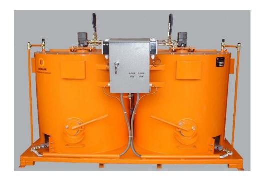
All Unimark vertical preheaters are supplied with powerful hydraulic motor driven agitators, with the pump driven by electric start diesel engines. The base mounting allows easy fitting to any vehicle or trailer. The burner system is designed to give very fast heat up time and is controlled by our electronic gas management system
