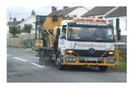
Unimark Truck Mounted Thermoplastic Road Marking Machines can be supplied as Spray, Extrusion, Raised Rib Profile Marking or a Combination Multi Mark Machine.
