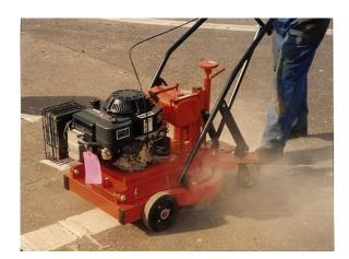
**Engine**: Kohler 13 HP vertical single cylinder gasoline engine. Smart choke easy
