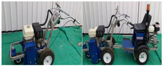
**Unirasor II Line Removal Machine** is the contractor choice for all-around scarifying jobs including Parking lot lines, intersection markings, construction zones and sidewalk smoothing. With the optional pusher system its productivity is unmatched and means you can get more work done every day without the fatigue from walking.
